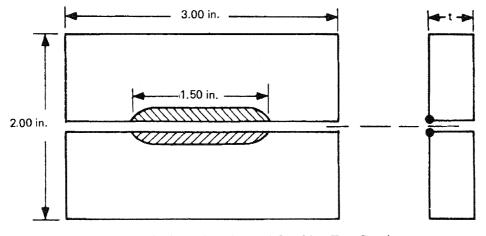
Longitudinal-Bead Underbead Cracking Test Specimen Figure X2-1
